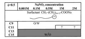
**Fig. 3** The effect on emulsion type of changing the hydrophobic tail length of n-alkyl carboxylate surfactants. The *question mark* domain corresponds to the emulsion-breaking region where emulsion type was found to be uncertain. C9, C11, C13 and C15 stand for m=9, 11, 13 and 15 in the above surfactant chemical structure
